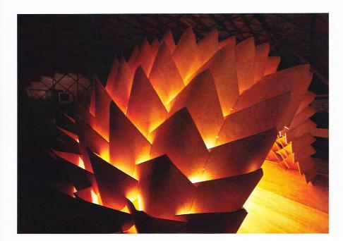
curved shape. Within six hours, these numbered shells are assembled by slotting them into place without using any plan drawings, glue, or screws. The underlying equilibrium surface geometry removes all internal forces and deformations from the pavilion, which becomes a self-supporting, freestanding, lightweight skin.
