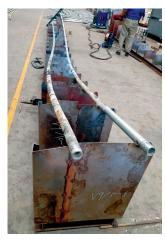
6 Two-dimensional bending using manual pipe-benders of pipes according to approximative planar curve projections [Program Contractors Ltd. (PCL) 2021 ©
