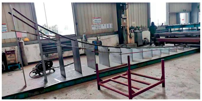
8 Three-dimensional bending using blowtorches of two-dimensionally bent pipes according to waterjet-CNC-cut steel jigs [Program Contractors Ltd. (PCL),
